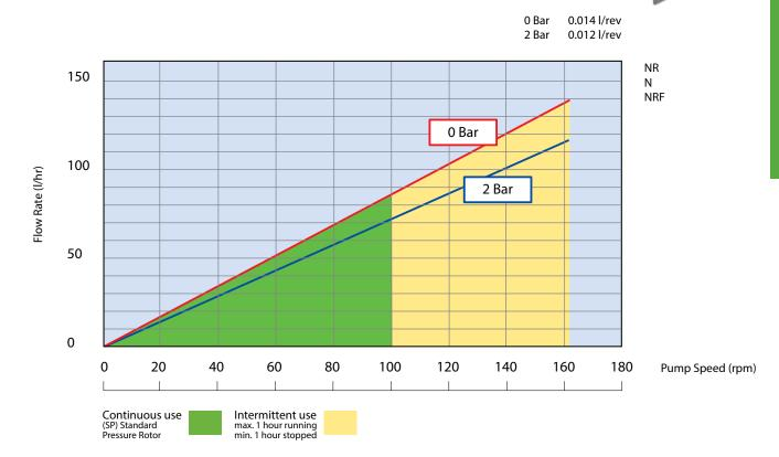
Flows are typical and were measured with water at 20°C with no suction lift or discharge pressure. Actual flows will vary according to suction conditions, discharge pressure and normal component production tolerances.
