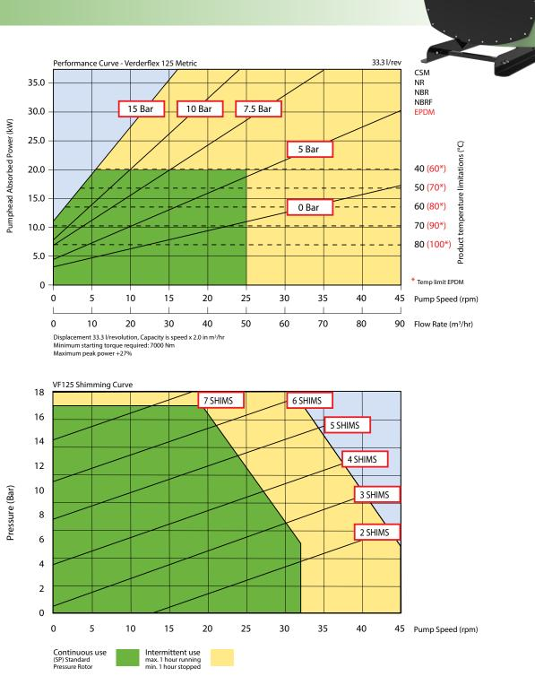
For product temperatures above 65°C and/or viscosity above 2000 mPas use one shim less than shown
