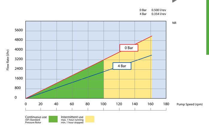
Flows are typical and were measured with water at 20°C with no suction lift or discharge pressure. Actual flows will vary according to suction conditions, discharge pressure and normal component production tolerances.
